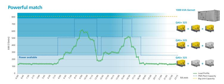
Note: this data is simulated. It's based on a typical industrial daily load diagram.
